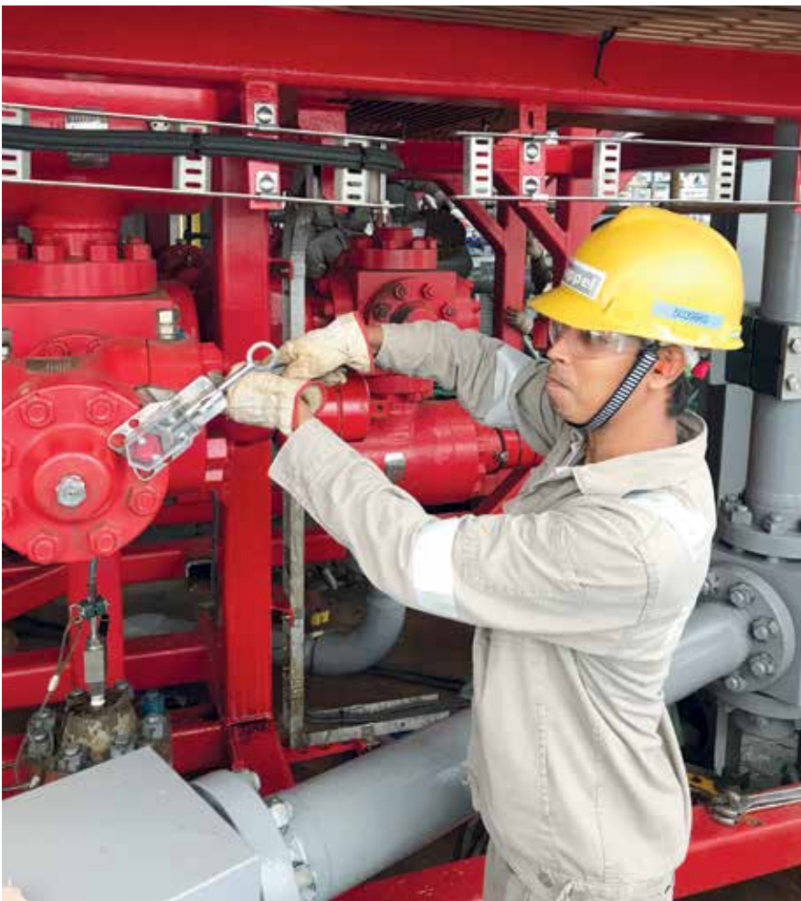
The newly developed tightener, which consists of a spring lock mechanism, reduces the risk of finger injury in constrained spaces especially onboard rigs and vessels
